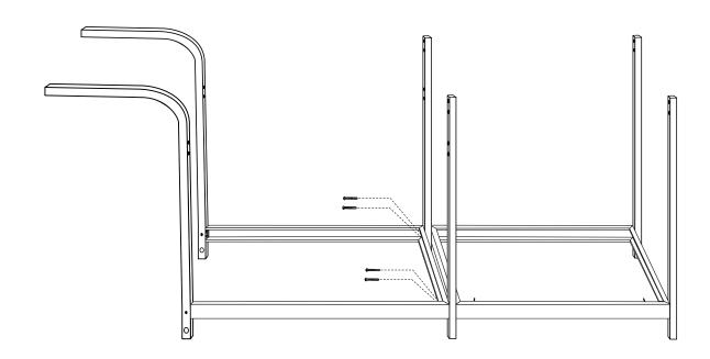
Attach tank support bracket to open end of grill bottom frame using two M6 X 35 bolts and M6 X 5 hex nuts.
